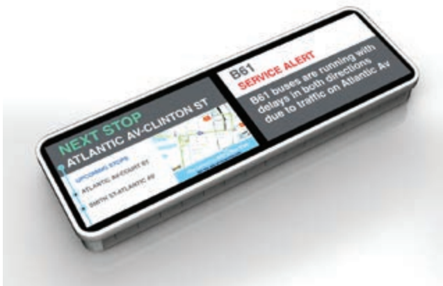
Fig.2. In the event of a disruption both screens of the TWIN display unit are used for passenger information purposes - left dynamic passenger info. and right the disruption notice!
