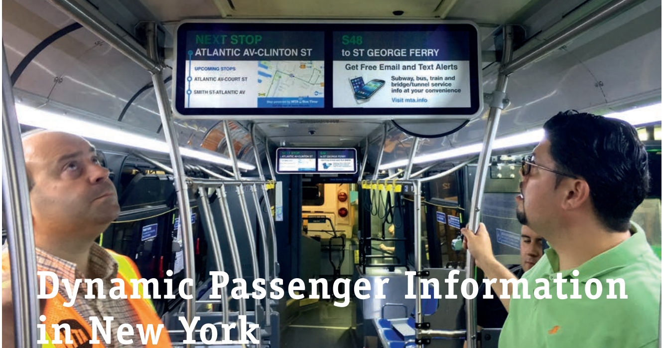
Image 1. The Nova Artic articulated bus is equipped with 3 ceiling-mounted dual display units ensuring both dynamic passenger information and entertainment are visible from all seating positions.
